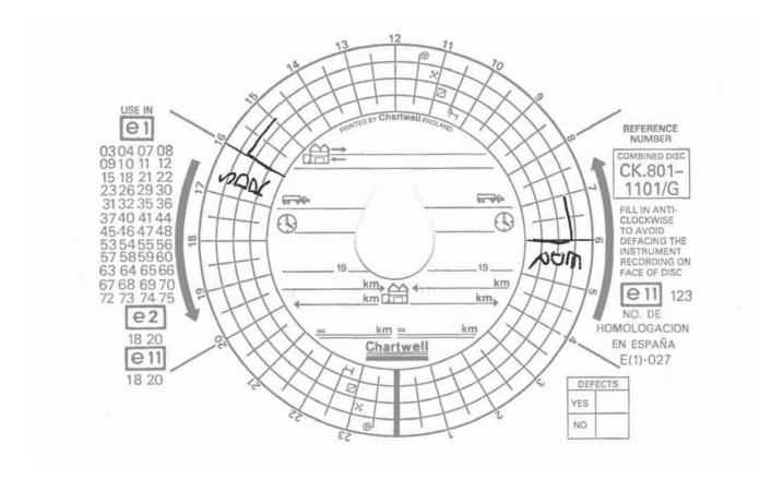
This is an example of manual entries made on the rear of a tachograph chart by a driver who started his day at 06.00 with an hour's work doing other duties away from his vehicle. He also finished his day with an hour of other work away from his vehicle and has indicated both the end and the start of a daily rest period. His activities while with the vehicle are recorded by the instrument on the other side of the chart once it has been inserted.
