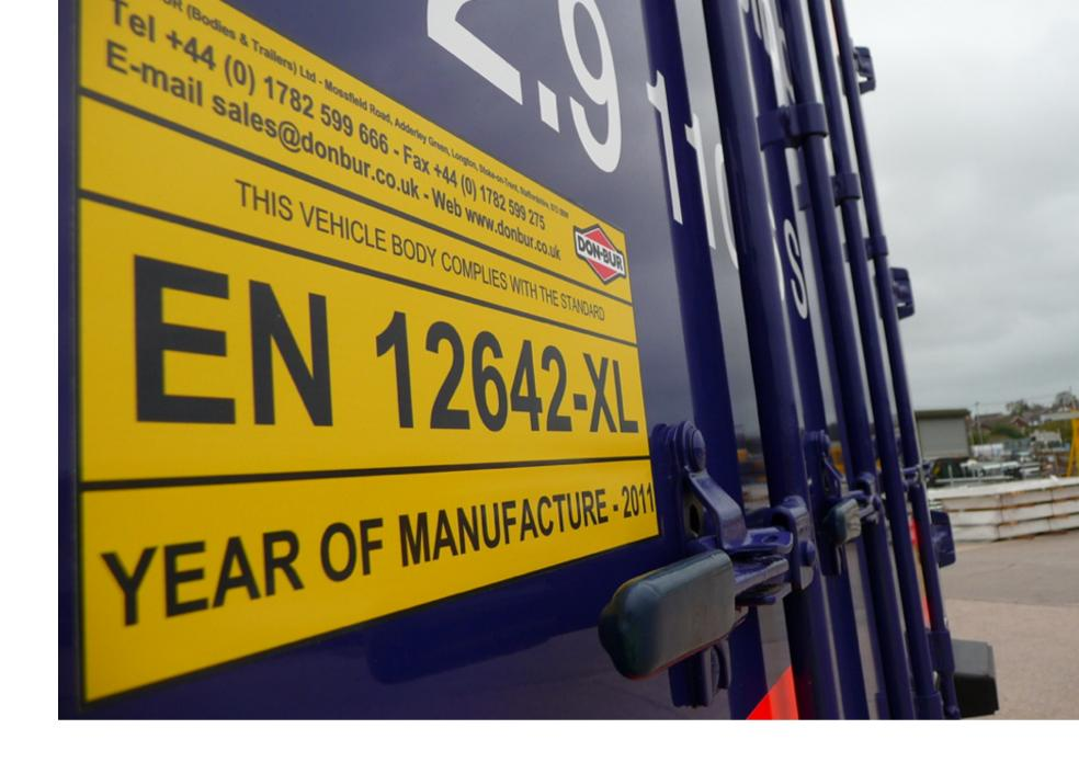
Trailers and vehicles that have been constructed to the EN 12642 XL standard are rated to withstand a minimum of 40% of the rated payload to the side, without additional load securing when used in accordance with the manufacturer's directions.
